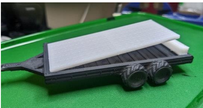
Figure 11: The 3D printed trailer prototype.
